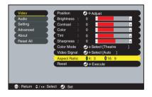
Press the [◄] and [►] buttons to set the aspect ratio to either "4:3" or "16:9", and then press the [Enter] button.
