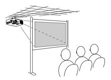
\* A special method of installation is required in order to suspend the projector from the ceiling. Please contact the place of purchase if you would like to use this installation method. The optional ceiling mount is required when installing the projector to the ceiling. (p.80)
