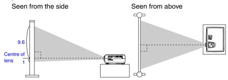
If it is not possible to set up the projector so that it is perpendicular to the screen, it can be set up at a slight vertical angle instead. You can extend or retract the front adjustable feet to adjust the projection angle within a maximum range of 10°.
